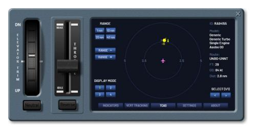
**Solid red square** – *resolution advisory* (RA). These Al-aircraft require a vertical flight maneuver (Up or Down) to avoid a collision. Removed at a distance of up to 5 miles with an altitude difference of less than 750 feet.
