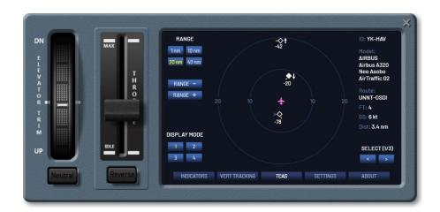
**Solid white-filled diamond** – *Proximate traffic.* Removed at a distance of between 10 and 15 miles with an altitude difference of 1,200 to 10,000 feet.
