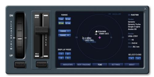
On the TCAS screen, there are buttons for changing the coverage range from 0.5 to 60 nautical miles, 4 display modes for selecting the amount of information displayed for each traffic object in the detection zone. Buttons for selecting a traffic object to get detailed information. You can also quickly select a traffic object by clicking on it.
