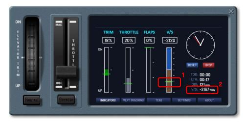
When the vertical speed indicator on the variometer is aligned with the marker (highlight 1 in the figure above), the aircraft will descend along the descent path of the active flight plan, as shown in the figure below.
